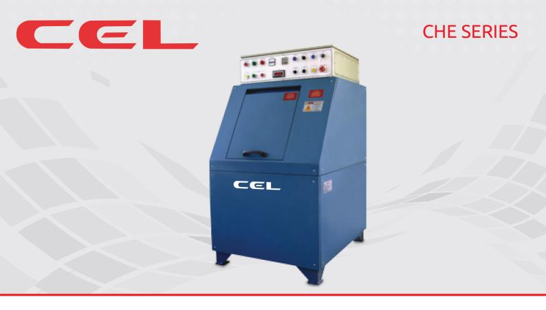
Centrifugal High energy machine is manufactured to meet the most rigid standards as demanded by specific industrial requirements of high volume and high surface finish. The machine generates a very high centrifugal force for extremely low process times. The machine is fitted with 4 hexagonal barrels with replaceable polyurethane lining. Sizes up to a maximum of 240 liter capacity are available with complete automated unloading mechanism.
